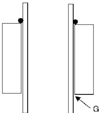
The optimum volume of brazing alloy required in a joint is 25% more than the volume of the joint gap at the brazing temperature.
